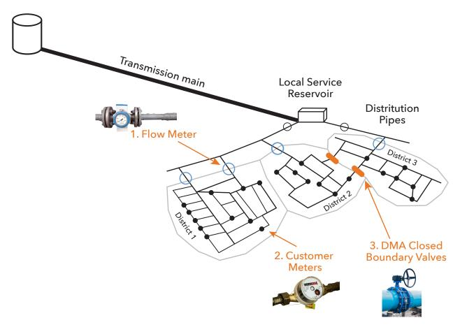
Traditional DMAs can also have adverse effects on both hydraulics (reliability and redundancy) and water quality (water age). A DMA limits supply reliability as it restricts water supply to customers through a single pipe at the DMA inlet. If
