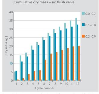
Figure 7. Cumulative mass of settling solids pumped out of the TOP sump in 12 pumping cycles for 3 operating stop-start level bands:0.0-0.7; 0.1-0.8; 0.2-0.9
