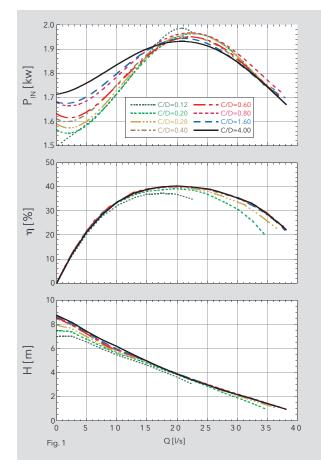
Figure 1. Effect of relative bottom clearance C/D on pump performance
