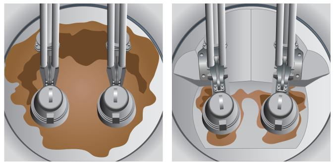
Figure 5. Back-to-back test - sand and plastic bead deposits (contour marked by a red line) in the standard and TOP sumps after a total of40 pumping cycles. The mass of sediment in the standard sump was 94kg and in the TOP sump, 4kg
