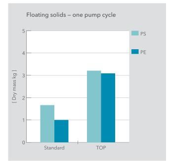
Figure 8. Mass of floating solids pumped out of the standard and TOP sumps in one pumping cycle; solids modeled by beads of polystyrene (PS) and polyethylene (PE)
