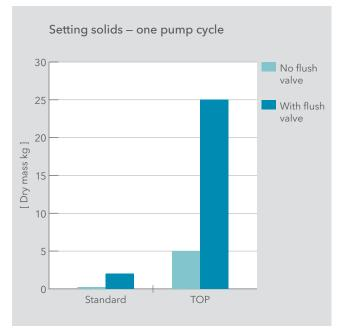
Figure 6. Mass of settling solids pumped out of the standard and TOP sumps in one pumping cycle
