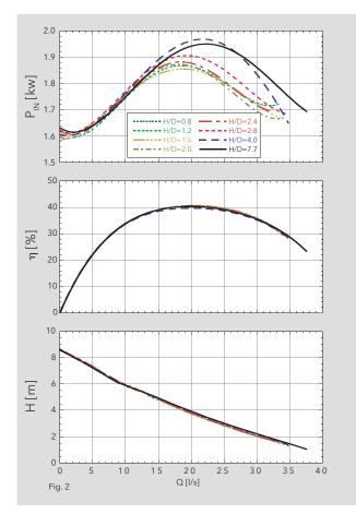
Figure 2. Effect of relative water depth H/Don pump performance
