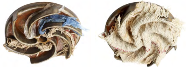
Figure 6 and 7: Accumulation in a vortex impeller
