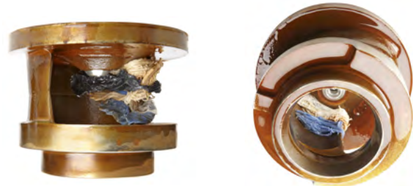
Figure 4 and 5: Accumulation in a single-vane impeller
