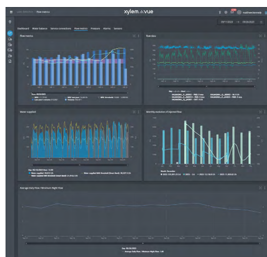
Meter Data Analytics captures, uploads, and displays meter readings, regardless of vendor, and alarms in a central, unified platform.
