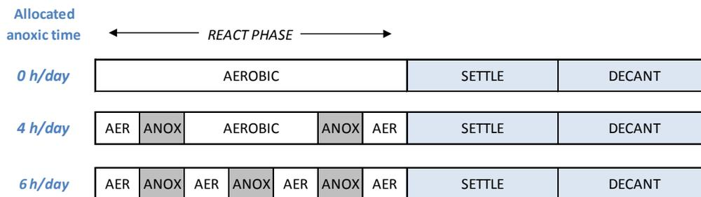
Figure 1- Treatment cycle configurations tested in the continuous feed SBR
