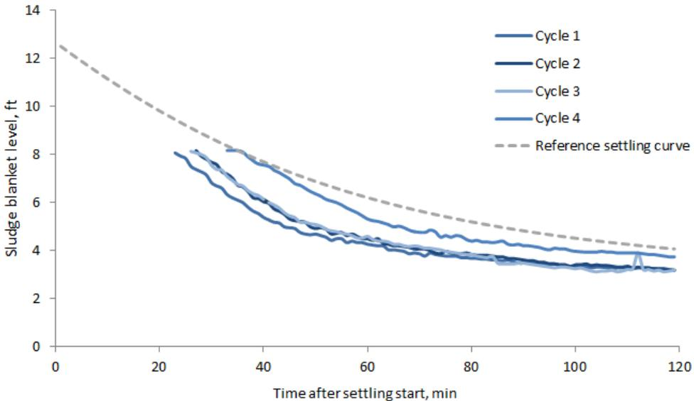
Figure 3 - Example of measured sludge blanket level during four treatment cycles compared to a reference settling curve based on the basin mass and SVI.
