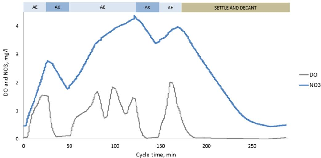
*Figure 2 - Online measured values of dissolved oxygen (DO) and NO<sub>3</sub> for the second treatment cycle configuration including two anoxic periods during the react phase. AE = Aerobic period, AX = Anoxic period.*
