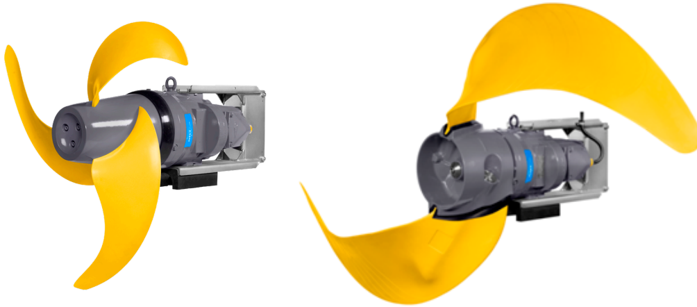
Figure 8. Left: mid-size low speed mixer suitable for oxidation ditches where reactor geometry does not allow for large, low speed mixers (Xylem Inc., 2012a). Right: large, low speed mixer highly suitable for oxidation ditches, capable of high thrust at low power input (Xylem Inc., 2012b).
