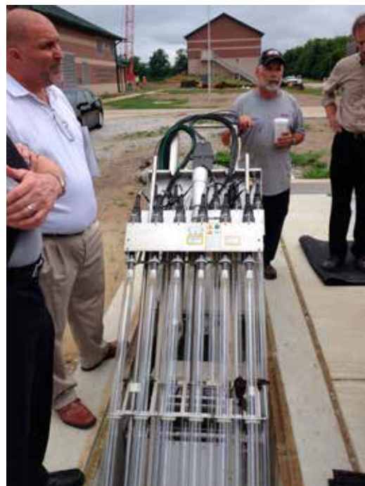
Autolift provides ease of access, for safe, quick maintenance
