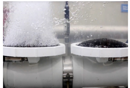
Clean versus dirty diffuser.
