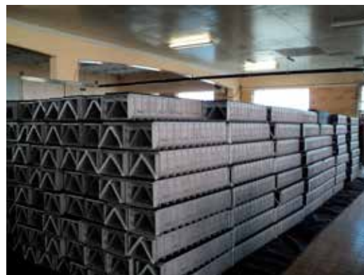
The Leopold Universal Type SL dual lateral filter system consists of 30 dual cell filters.
