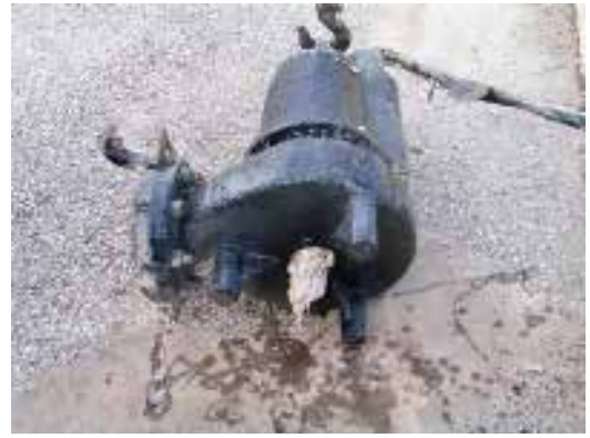
Flygt N pumps eliminated the frequent clogging problem caused by the former pumps
