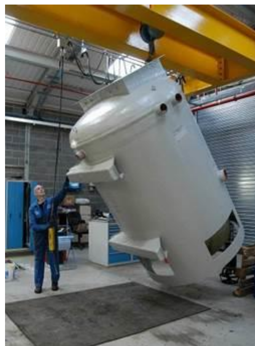
Prefabricated Flygt TOPS packaged pump station, fully kitted out with pumps, valves and pipework, delivered to site and simply placed in the ground: Minimizing civil engineering and mechanical and electrical works on site to allow for quick installation and reduced project lead times.
