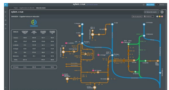
Water catchment and adduction processes in EMASESA
