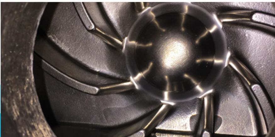
THE COMAG SYSTEM'S MAGNETITE BALLAST EXTENDS EQUIPMENT SERVICE LIFE. THIS IMPELLER PUMP HAS BEEN OPERATING CONTINUOUSLY WITH THE COMAG SYSTEM FOR MORE THAN A DECADE WITHOUT ANY SIGNS OF ABRASION.
