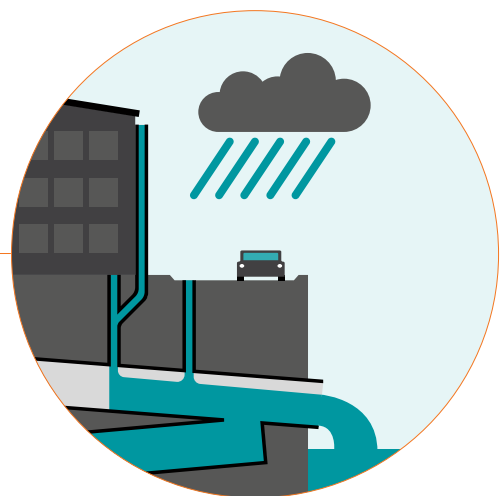
Combined Sewer Overflow (CSO)
