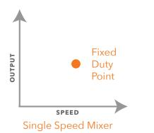
A single-speed mixer has a fixed output that does not allow for a change, even if the process demand were to increase or decrease.
