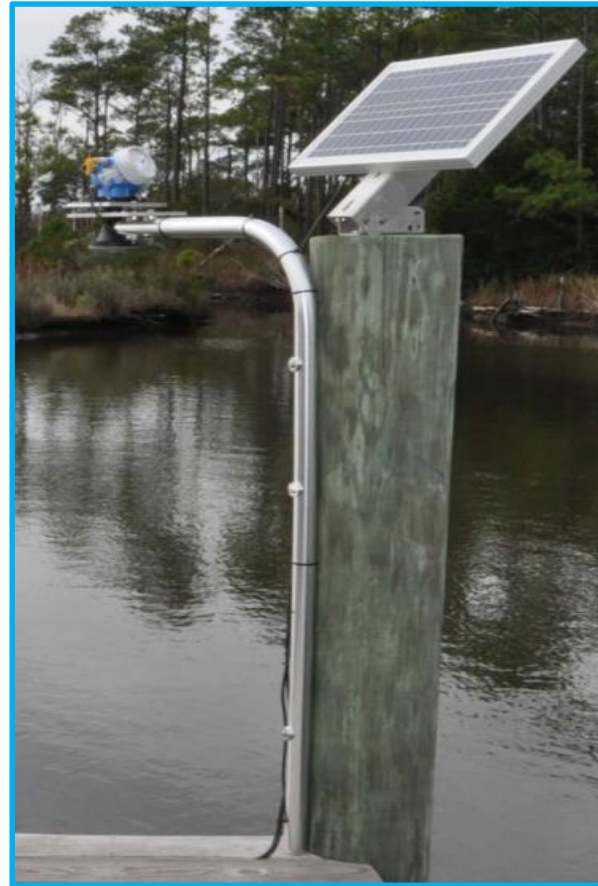
Tide Station Radar Level Sensor
