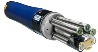
The YSI ProDSS is an ideal instrument for environmental spot-sampling, while the YSI EXO sonde platform is perfect for continuous environmental monitoring.
