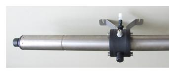
len key size 6, somewhat tighten the Allen screws langes to the measuring chamber so that the meapher cannot easily be moved on the spectral seneaded connection of the spectral sensor must still and completely visible through the knurled and amp-connection of the measuring chamber.
