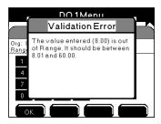
Autofix occurs when a high or low control value is entered that breaches the set point value. Autofix changes the high or low control value by one least significant digit away from the set point value. The set point value is never adjusted.
