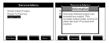
2. at Run Screen to proceed with Output Test. Output Test Menu opens:
