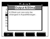
4/20mA menu configuration information is provided at AquaManager Help. See AquaManager Help contents>working with nodes>expansion modules>ioem expansion module>configure ioem 4mA-20mA output to a 5X00 system bookmark. Configure 4/20mA outputs at sensor system tabs in AquaManager. 4/20mA configuration fields are located at the bottom of all sensor system tabs.
