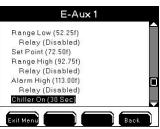
Control relays configured in the Set Point control mode energize when a user configured control value is received from the input device and is processed by the 5200A.
