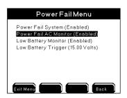
Disabling the Power Fail System will disable AC power events and disable the General Alarm in the event of low battery for DC power. **Disable** Power Fail AC Monitor when powering 5200A by DC power source.
