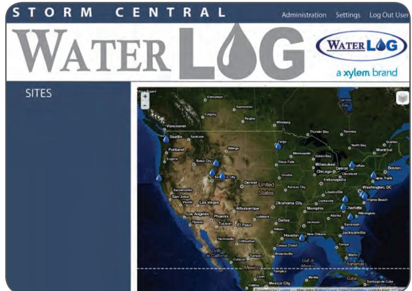
Sites using GOES to transmit their data can also be set up within Storm Central to have their data retrieved, decoded, and made easily accessible. Both WaterLOG ASCII (SHEF) and Pseudo-Binary formats are fully supported.
