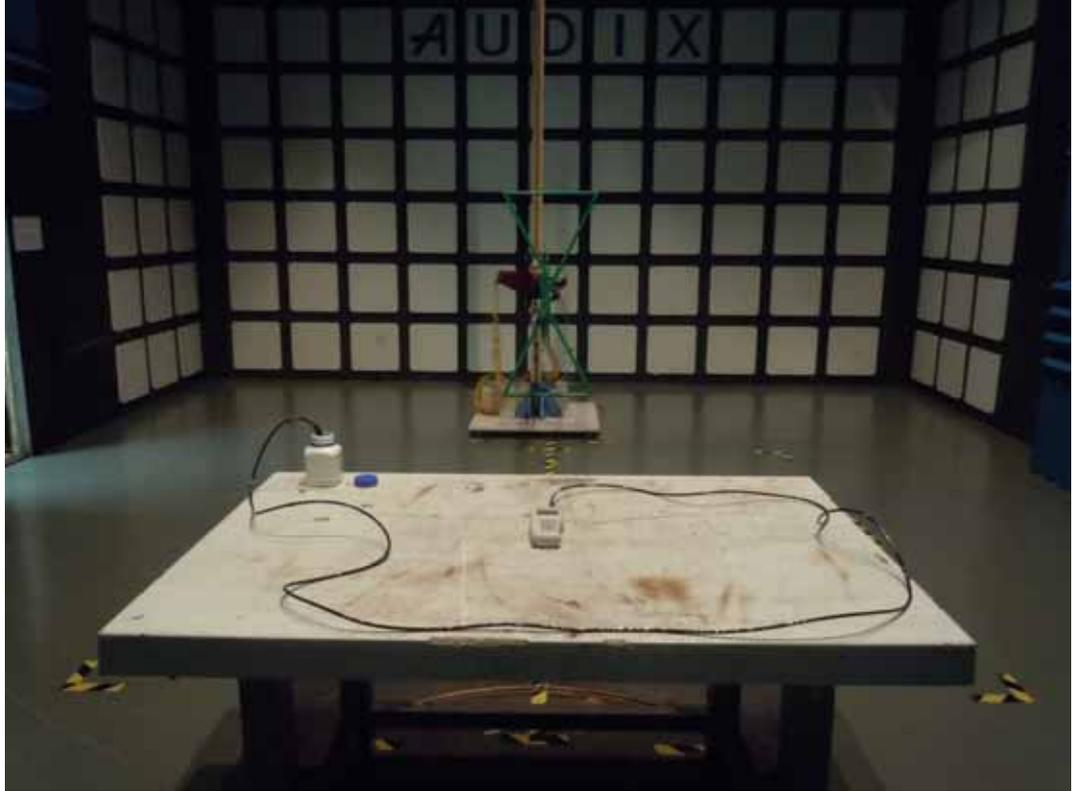
*FRONT VIEW OF RADIATED EMISSION TEST*
