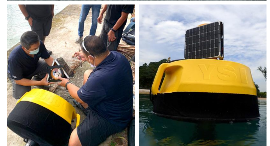
Figure 2: DB600 buoy deployed at Bendera Bay, St. John's Island, Singapore. Onsite training to SJNML - TMSI staff on installation, deployment and maintenance of DB600 buoy and YSI EXO3 Sonde.
