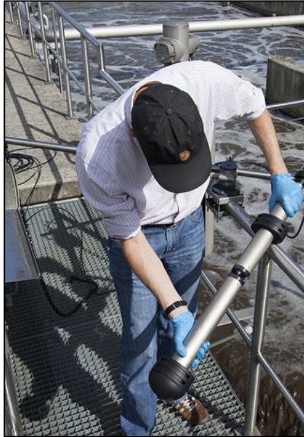
July 7 Online Wastewater Monitoring of COD/BOD With Spectral Sensors
