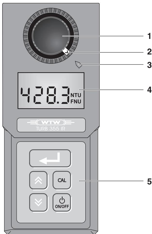
**1** Cuvette in the cuvette shaft
