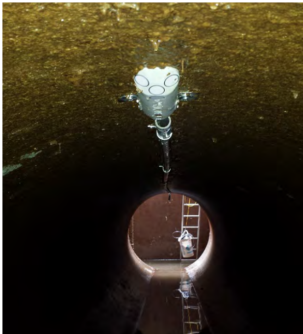
The SonTek-IQ Pipe is intended as either a bottom or top mounted flow meter that can be used in most industrial or agricultural applications. It can provide accurate flow values in pipes from 0.5m all the way to 5.0m, independent of whether these pipes are full or not.
