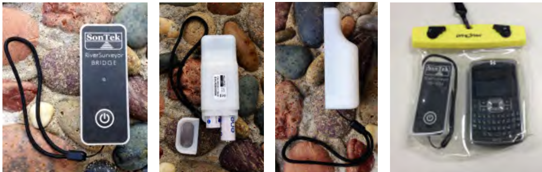
Figure 190. SonTek Communications Bridge and mobile (far right) in supplied dry bag.
