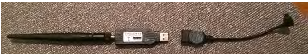
Figure 204. Connecting MicroUSB to USB adapter to SonTek Radio Dongle
