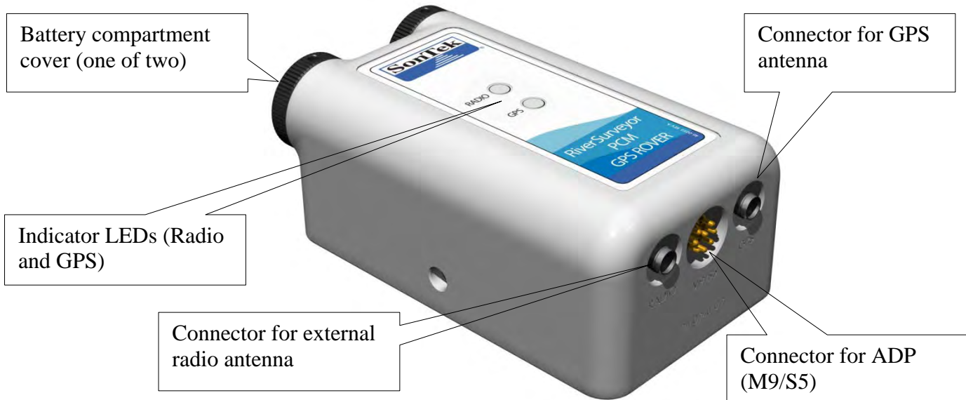
Figure 196. Configuration B – PCM DGPS. Figure shows the PCM and its main components.
