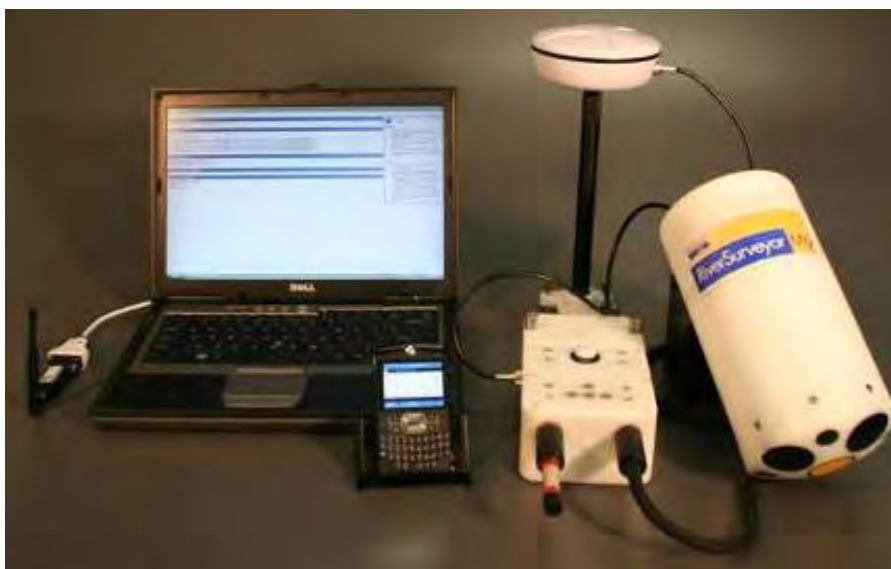
Figure 16. Hardware for RTK GPS Option with Bluetooth Communications. Note BT Dongle requires power from a second USB port (not shown).
