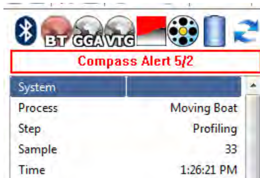
Figure 40. Compass Alert box shown. In this case there have been 5 samples with magnetic error >3.5% and 2 samples with greater pitch and/or roll value than experienced during calibration.
