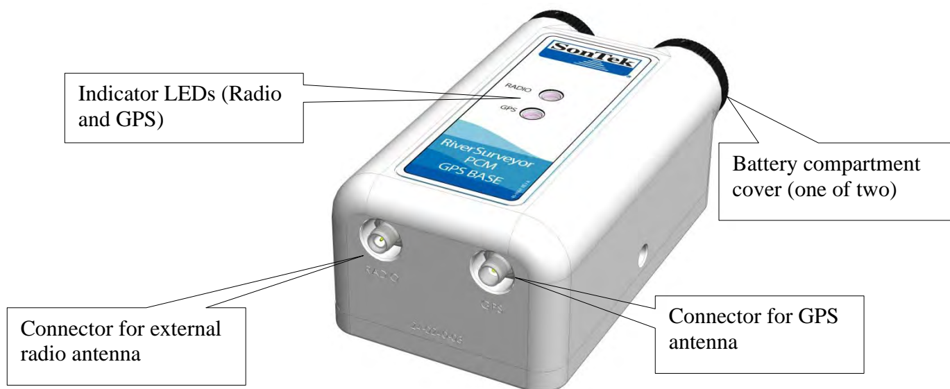
Figure 199. Configuration C – PCM RTK-GPS (Base). The Figure shows the RTK Base Stations and its components.
