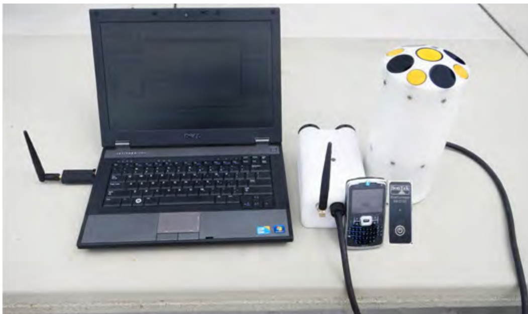
Figure 195. Configuration A – PCM (Telemetry Only). Figure shows the different methods of connecting to the PCM: Via mobile phone (through Bridge), or through PC (via radio dongle on the left of the image).
