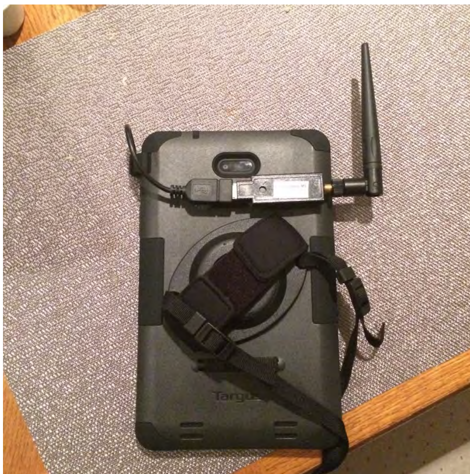
Figure 205. Securing the adapter and USB dongle to the tablet
