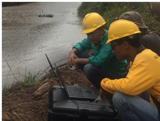
Use of the Sontek M9 to collect discharge and cross sectional data to better understand canal water routing
