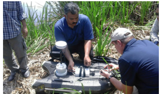
Suneesh Nair, Application Specialist, Sea and Land Technologies and Justin Stockley, AP Xylem Surface Water, demonstrate the SonTek M9 for canal discharge measurements and bathymetry.
