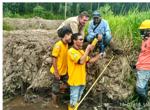
Use of the Sontek M9 and Hypack software to collect bathymetric data at Baung, Palembang for a navigable section of the river leading to the Paper Mill jetty.
