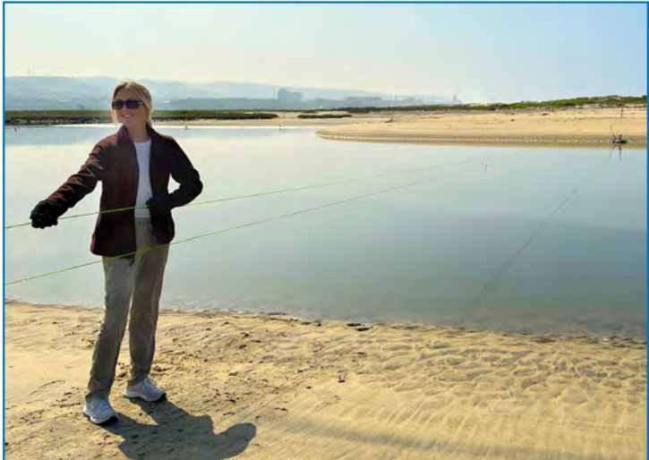
SDSU student Callie Summerlin conducts a transect measurement with the SonTek-RS5. The process was conducted by various members of the survey team throughout the entire tidal cycle to assess the flow of water (and pollutants) within the estuary.
