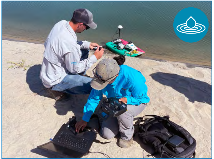
In one of the first site studies conducted in 2023, SonTek’s Matt Klipfel and Dr. Xue Fan use the SonTek-M9 to conduct the first bathymetric survey that was used to examine scour of the river mouth to develop a bathymetric baseline to compare to satellite imagery to infer suspended sediment load.
