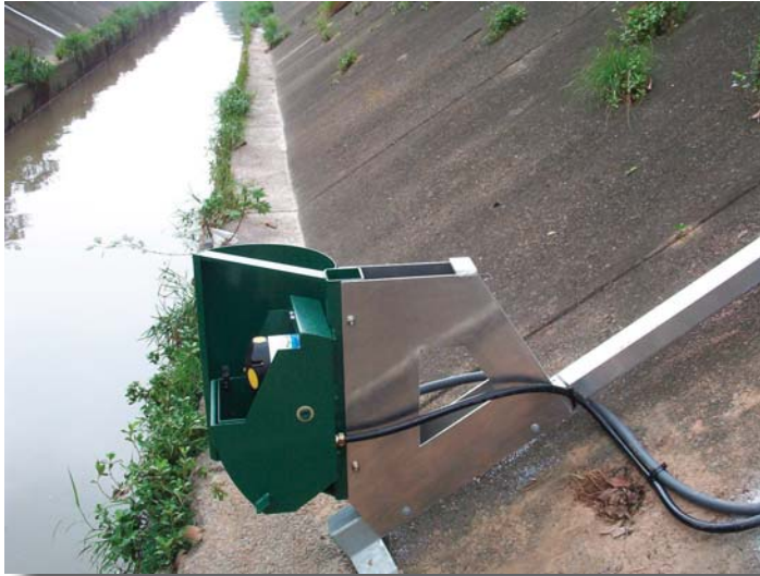
Innovative “Knights Head” stations use automatically retracting hoods to protect SonTek Argonaut current meters.
