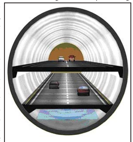
Kuala Lumpur's SMART tunnel diverts traffic as well as floodwater under moderate-rain conditions. If deluges persist, operators can close the tunnel and flood the roadways for greater water-holding capacity.
