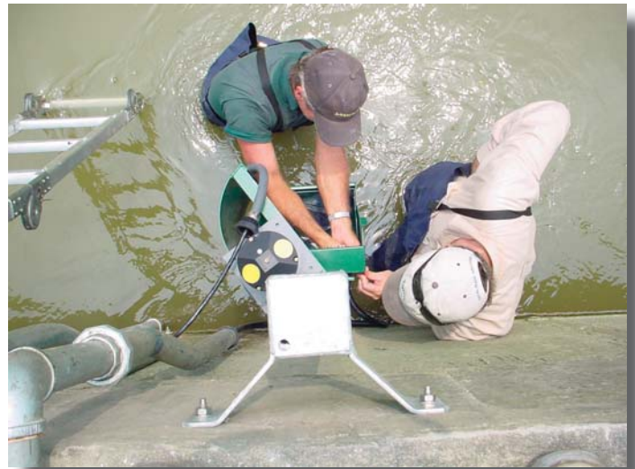
The Greenspan team installed 16 SonTek Argonaut acoustic Doppler current meters at carefully determined heights to measure current and depth during floods with extreme accuracy.
