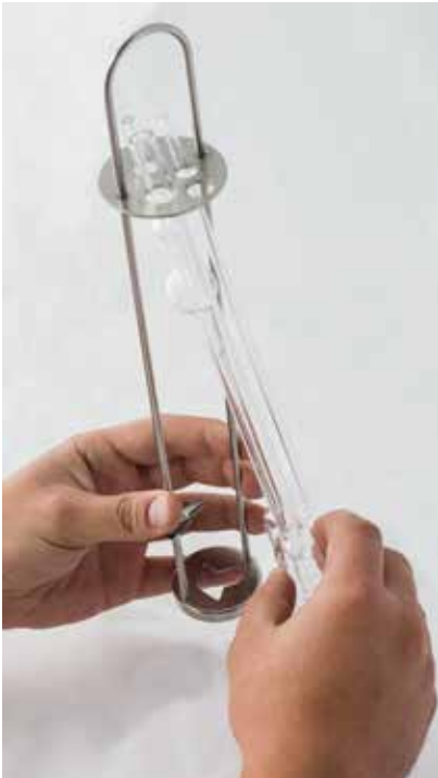
Fig. 14 Using the viscometer in a bracket
