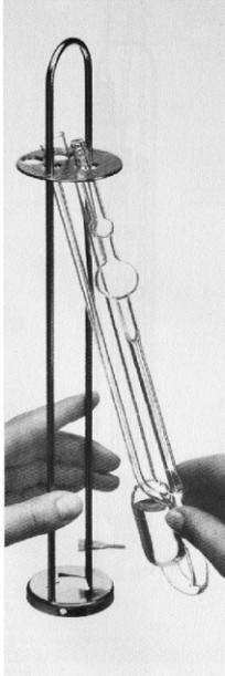
**Fig. 4** Inserting or replacing a viscometer with light-barrier sensing
