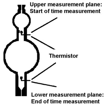
**Fig. 2** Viscometer for thermo-resistive measurements
