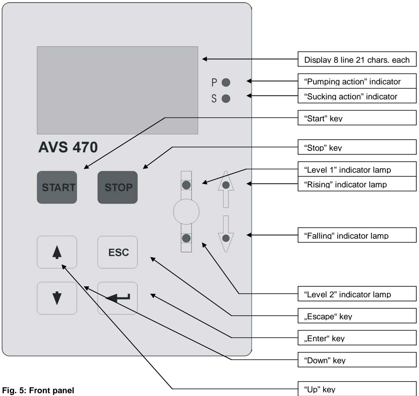
Fig. 5: Front panel
