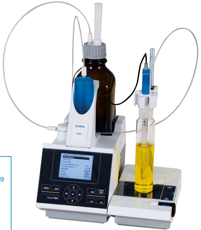
Titration application “chemical oxygen demand” COD
