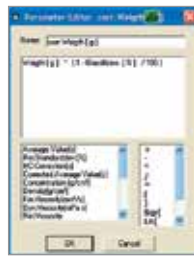
All the important parameters required for the measurement are displayed on the "Methods/Results" page. If necessary, the parameter editor can be called up using "Add Parameter", in order to enter non-standard or customer specific formulae.
