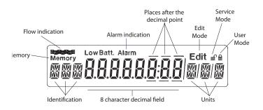
The multi-function display shows the eight-digit meter reading, along with symbols and short texts for user operation purposes.
