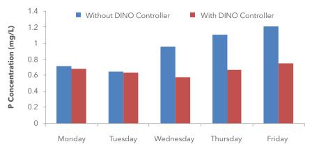
Without DINO controller, one treatment plant experienced phosphorous spikes 2-3 days per week due to large nutrient returns to the main plant from solids processing (i.e. dewatering digested biosolids). Implementation of the DINO controller reduced the returned nutrients, resulting in greater stability and ensuring permit compliance every day.
