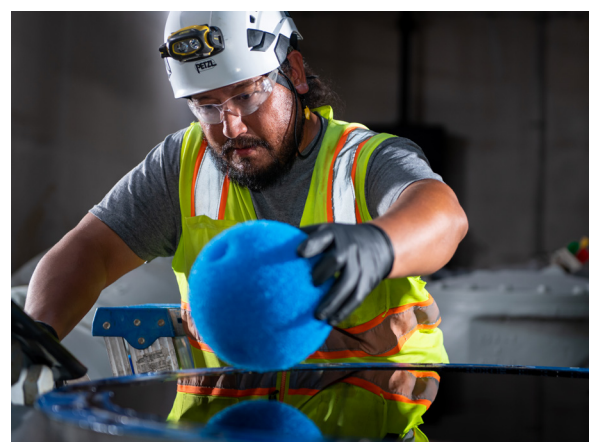
SmartBall inline free-swimming pipeline inspection platform
