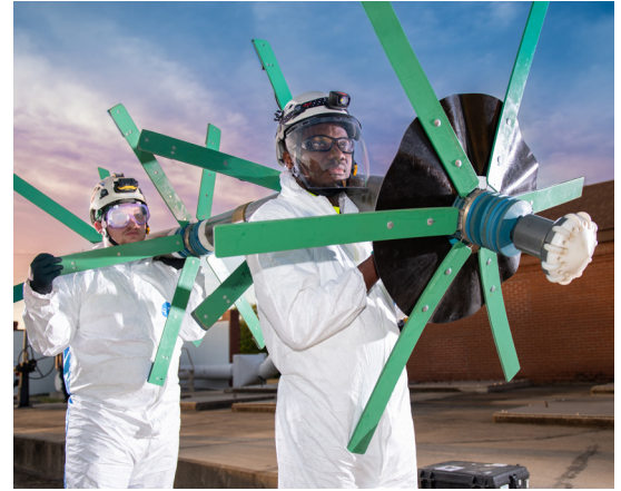
PipeDiver inline free-swimming pipeline inspection platform
