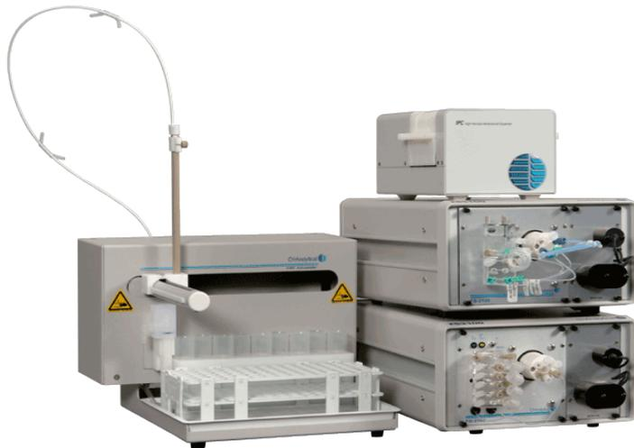
FS3100 Introduced 2006, Versachem cartridge with snap on and off chemistries, 2 channels of FIA and 3 channels of SFA.
