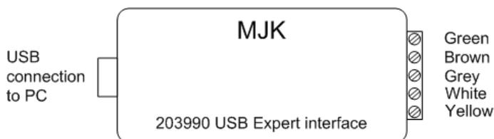
**NB: For Expert™ 3400 only:** 203990 PC Interface used for connecting Expert™ Hydrostatic Level Transmitters to a PC using Expert Link.
