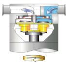
Fluid enters inlet port and is drawn through inlet check valve when piston moves away from the check valve assembly.
