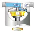
As piston moves toward the check valve, the fluid is forced through outlet check valve and out of the pump.
