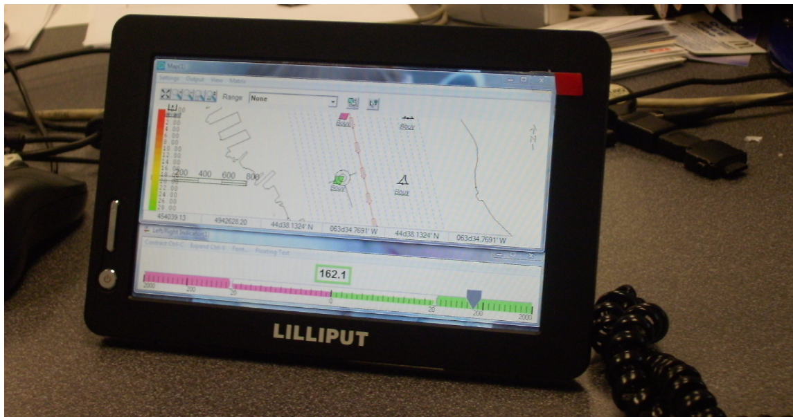
FIGURE 2. Screen Configured with HYPACK® SURVEY Map Window and Left-Right Indicator
