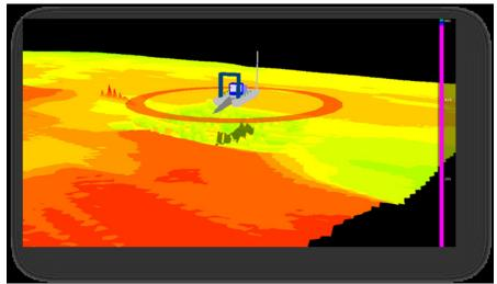
determine the current bottom. The boring samples determine the depth of the contaminant so there are two depths: a current bottom and a contaminant depth. Both of these depths are then taken into the TIN MODEL program to create separate matrix files.
