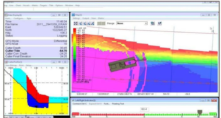
DREDGEPACK® installed on a cutter suction dredge with a carriage spud. Note the real-time cross section that is taken along the arc of the cutter head!
