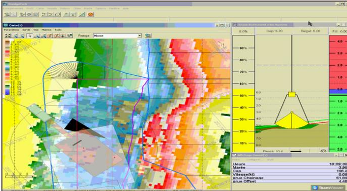
DREDGEPACK® provides the solution to track the depth and position of the bucket on a clamshell dredge.
