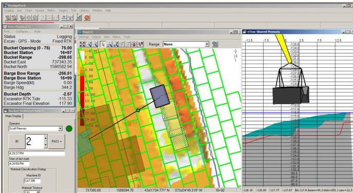
Proposed bucket patterns for a crane or bucket operation can be generated in advance. DREDGEPACK® also keeps a history of bucket drops/placements for your reports.
