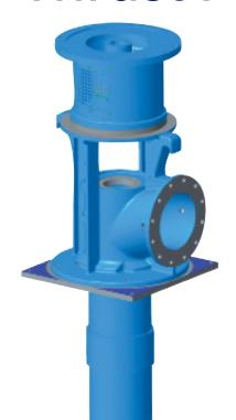
Thrust pots are required on vertical turbine lineshaft pumps using IEC motors which will not carry axial thrust loads. The thrust pot is installed between the discharge head and the motor.
