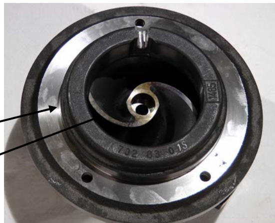
Figure 20 Locating insert ring on impeller
