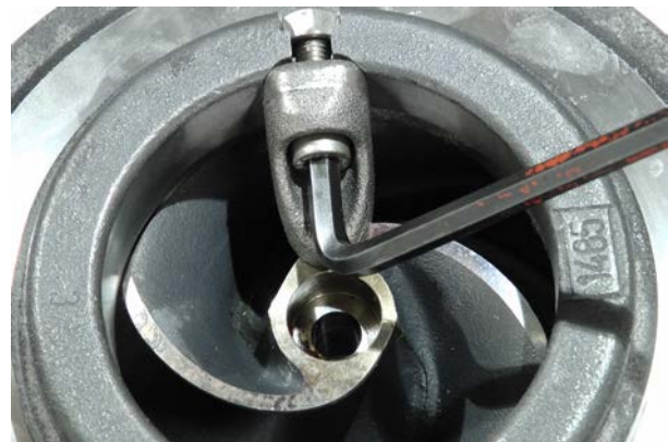
Figure 25 Tightening the cap screw with Allen wrench
