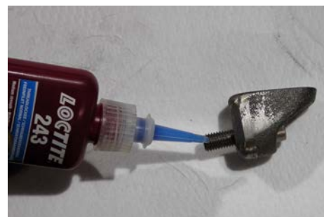
Figure 22 Applying non-setting thread lock compound
