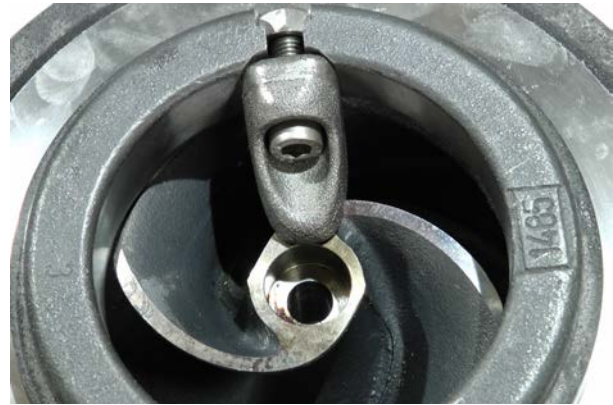
Figure 24 Aligning the guide pin lip with the centre boss of the impeller
