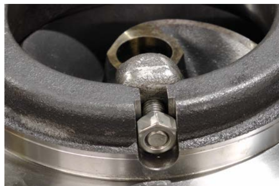
Figure 23 Locating guide pin assembly into insert ring
