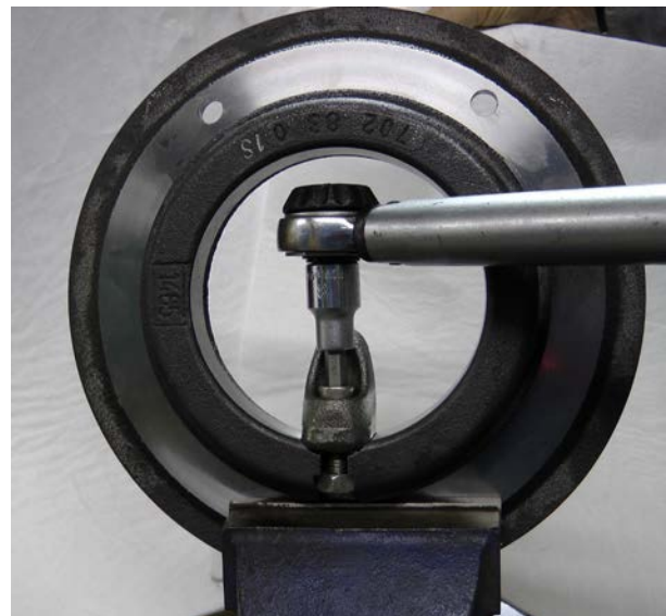
Figure 26 Tightening the cap screw with torque wrench
