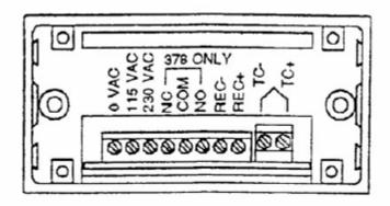
Wiring diagram Drawing 4
