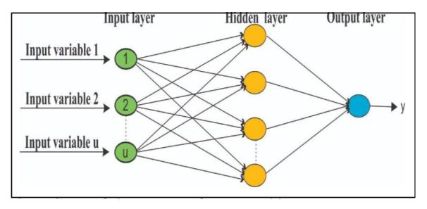
Figure 1: Layer structure of an ANN model
