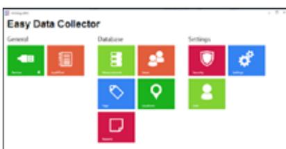
The evaluation software EDC (Easy Data Collector) is a self-contained, windows-based application software. It offers the collection, evaluation and storage of measurement data gathered with the TLC 750 NFC, especially to customers who don't need the MyCCP software. EDC focusses entirely on the measurement data, similar to the Winlog.basic.
