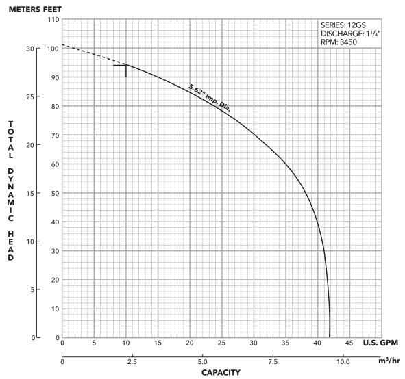
$\square$  = A 1½" minimum discharge pipe requires a minimum flow of 10 gpm to maintain a 2 ft./sec. scouring velocity. Flows less than 10 gpm will allow solids to settle in the pipe.
