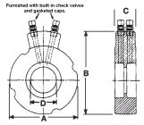
Maximum working Pressure 300 PSIG (2069 kPa) Maximum Operating Temperature 250°F (121°C)
