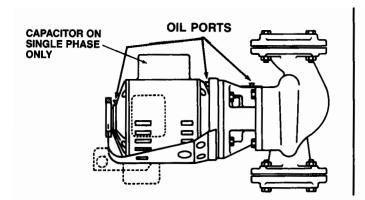
**NOTE:** The position of the conduit box is determined by the model of the motor used and must be positioned on the bottom or the side of the motor housing. As shown to the left.
